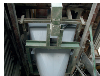
Photo 2, Dosing hopper for cement.
