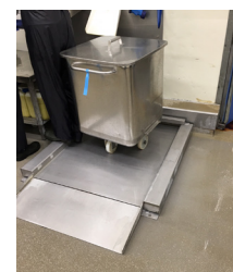
Photo 4. A weighing platform for weighing raw materials.
