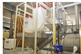
Photo 2. The input into the process of smaller components, supplied in big bags.
