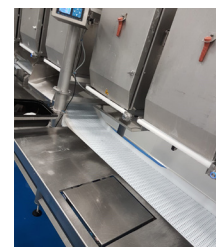
Photo 6. A built-in weighing system for manual dosing.
